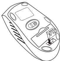
Fig. 6. Fitting the receiver into the mouse case
