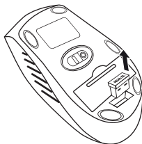
Fig. 7. Extraction of the receiver from the mouse case
